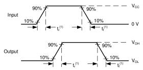
A. t<sub>t</sub> is the greater of t<sub>r</sub> and t<sub>f</sub>.
