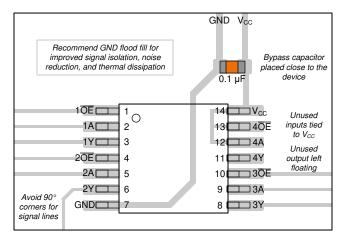
Figure 11-1. Example layout for the CD74HC126
