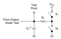
A.  $C_L$ = 50 pF and includes probe and jig capacitance.
