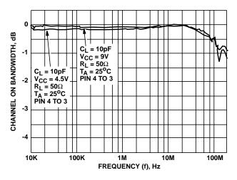
FIGURE 3. SWITCH FREQUENCY RESPONSE
