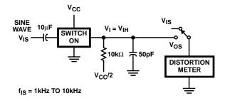
FIGURE 6. FREQUENCY RESPONSE TEST CIRCUIT
