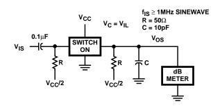
FIGURE 8. CONTROL-TO-SWITCH FEEDTHROUGH NOISE TEST CIRCUIT
