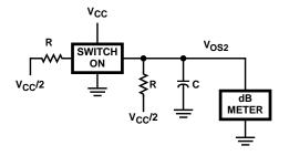
FIGURE 5. CROSSTALK BETWEEN TWO SWITCHES TEST CIRCUIT
