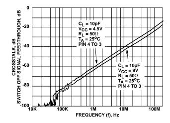
FIGURE 4. SWITCH-OFF SIGNAL FEEDTHROUGH AND CROSSTALK vs FREQUENCY
